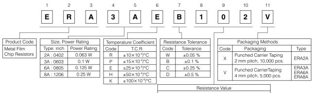
Consist of three figures for E24 series resistance value. The first two digits are significant figures of resistance and the third one denotes number of zeros following. (example) 102 :  $1 \text{ k}\Omega$
